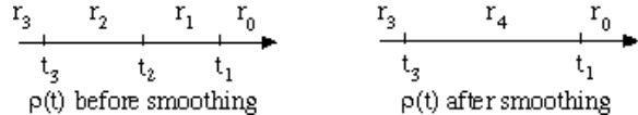
Figure 1: Smoothing fluid events over a link latency time. r_4 = (r_1(t_2 - t_1) + r_2(t_3 - t_2))/(t_3 - t_1) . Passage of time should be read right-to-left: t_1 < t_2 < t_3 .
